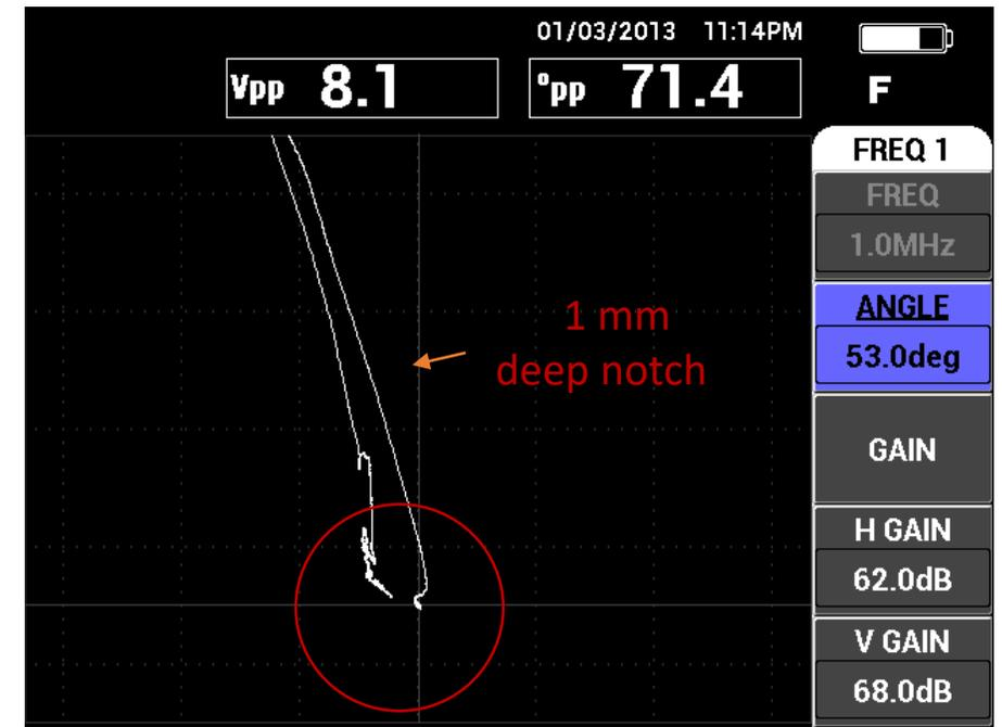
Noise caused by weld roughness
