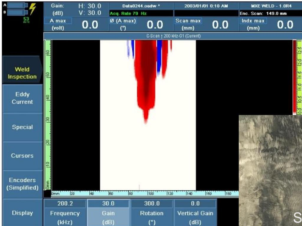
Stainless steel 304 C-scan image with 1/8 in. (3 mm) liftoff
