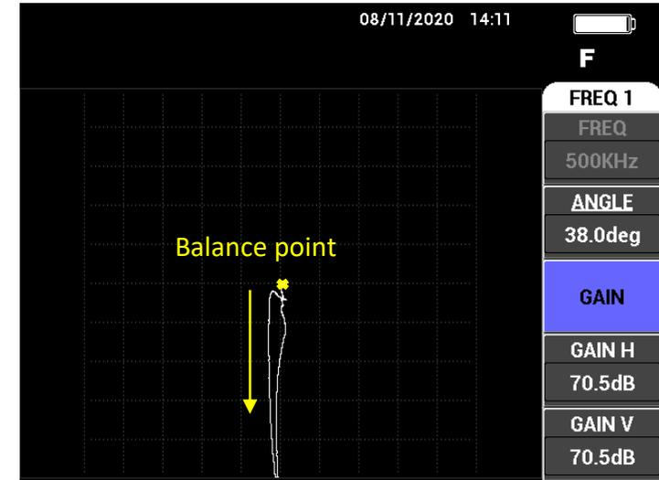
The impedance plane is unbalanced compared to the flawless area. The signal tends to move downward.
