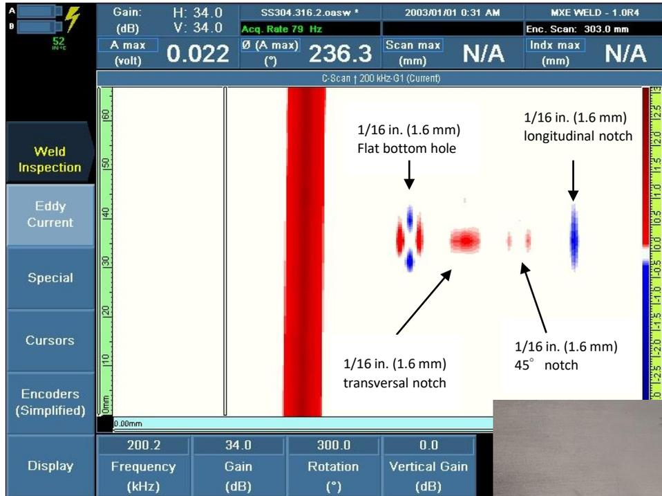
Stainless steel 304, C-scan image with 3 mm of lift-off
