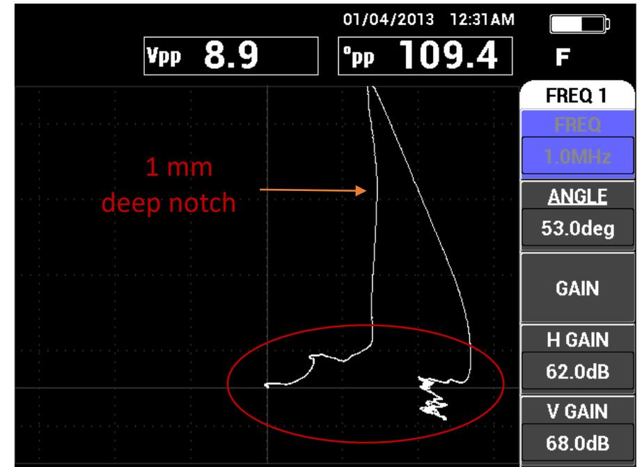
Noise caused by weld roughness
