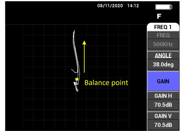
The impedance plane is unbalanced compared to the flawless area. The signal tends to move upward.
