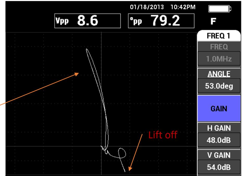
The gain was reduced by 14 dB to be able to see the entire crack signal on the screen.
