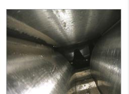
Inspect gear teeth and bearings for defects from wear and erosion, including color change and pitting
