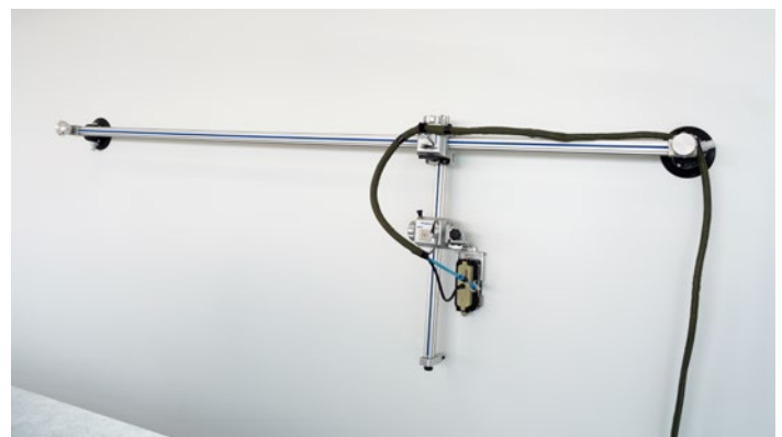
Semiautomated inspection using the 72-inch (1.8 m) long GLIDER scanner and OmniScan flaw detector
