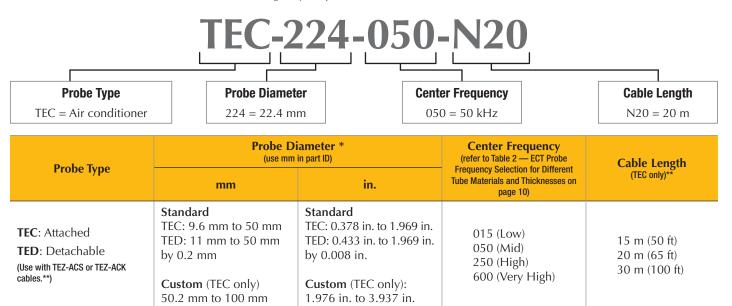
\*Refer to Table 1 — ECT Probe-Diameter Selection Guide for Common Tube Sizes on page 7 for assistance with probe diameter selection. \*\*TEZ cable information for TED probes is available on page 11.
