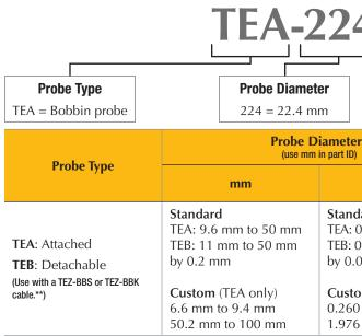
\*Refer to Table 1 — ECT Probe-Diameter Selection Guide for Common Tube Sizes on page 7 for assistance with probe diameter selection. \*\*TEZ cable information for TEB probes is available on page 11.
