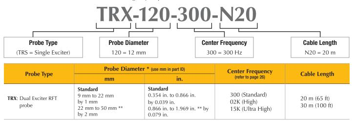
\*Refer to Table 3 — RFT Diameter Selection for Common Carbon Steel Tube Sizes on page 25 for assistance with probe diameter selection.
