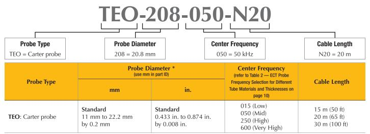
\*Refer to Table 1 — ECT Probe-Diameter Selection Guide for Common Tube Sizes on page 7 for assistance with probe diameter selection
