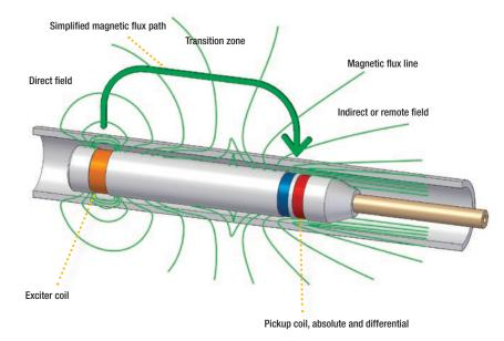
• The distance between the pickup and exciter coils is 2.5 to 3 times the tube OD. (Single exciter model shown.)
