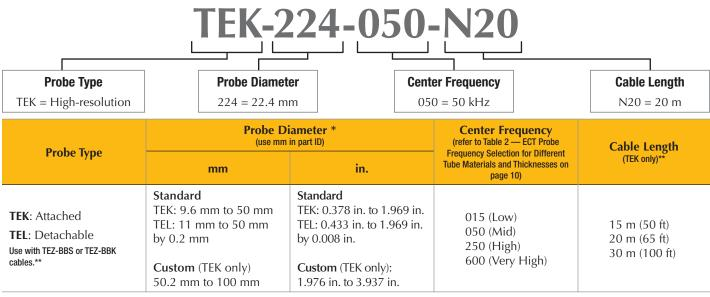
\*Refer to Table 1 — ECT Probe-Diameter Selection Guide for Common Tube Sizes on page 7 for assistance with probe diameter selection \*\*TEZ cable information for TEL probes is available on page 11.
