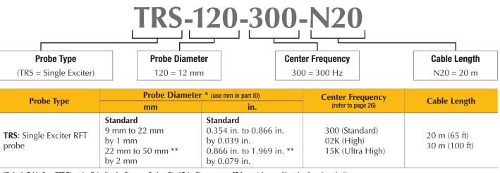
\*Refer to Table 3 — RFT Diameter Selection for Common Carbon Steel Tube Sizes on page 25 for assistance with probe diameter selection. \*\* Probes with a diameter greater than 26.0 mm (1.023 in.) have a lightweight design and probe body made of plastic and two stainless sleeves (see picture above).
