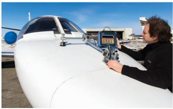
Zero-degree inspection just became even more accessible with the arrival of the OmniScan SX. For corrosion or composite inspection, Olympus offers field-proven solutions for detection of anomalies or wall loss.
