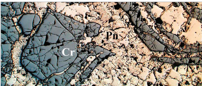
Digital photo-micrographs taken with an Olympus cross-polarized microscope showing chromite in nickel sulfides
