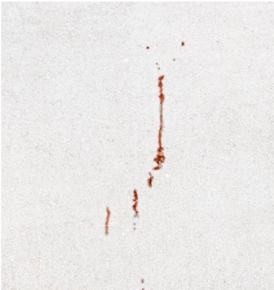
Red dye penetrant indications
