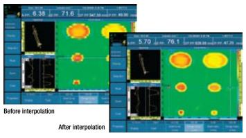
When working with two frequencies, a MIX signal can be generated to remove unwanted signals (for example; lift-off, fastener signals, etc.).
