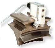
Shell inspection – This application demonstrates a single-rotation 100% inspection of small ammunition shells; the probe shown here is part of a small automated system that loads, inspects, and sentences each shell.
