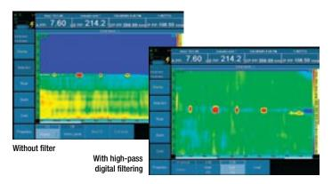
Several filters can be applied to the data such as high-pass, low-pass, median, and averaging. The figures above represent an application where the cracks are located at the edge of a lap joint, which has a sharp thickness variation. The filtered data can improve detection, especially for small cracks.
