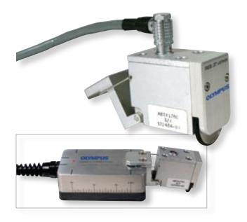
This encoder is built with an aluminum casing and a stainless steel wheel, and has a resolution of 27.1 counts per millimeter (688 counts per inch). It can be used with all standard ECA probes with the exception of the SBBR-026-300-032 and SBBR-022-300-032.
