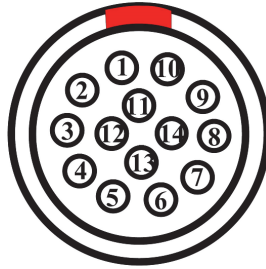
Figure 6-2 Alarm and I/O LEMO connector (contact view)
