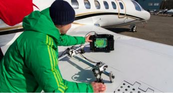
Encoded system: any two-axis encoding scanner can be used to inspect a part. Olympus offers two options: the GLIDER™ scanner, which is well-suited for flat or slightly curved surfaces, and the WING<sup>™</sup> scanner, which is specially designed for scanning curved parts (e.g., aircraft fuselages) and can even be used upsidedown due to its Venturi vacuum-cup system. For more versatility, a handheld one-axis encoding scanner, equipped with an Indexer Clicker, is also compatible with this system.
