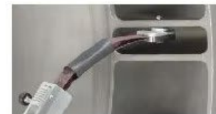
86PR-3 Low-profile Articulating Probe
