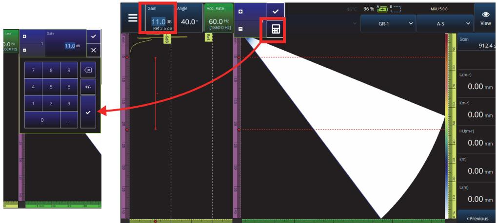
Figure 2-9 Parameter adjustment using up/down arrows or keypad
