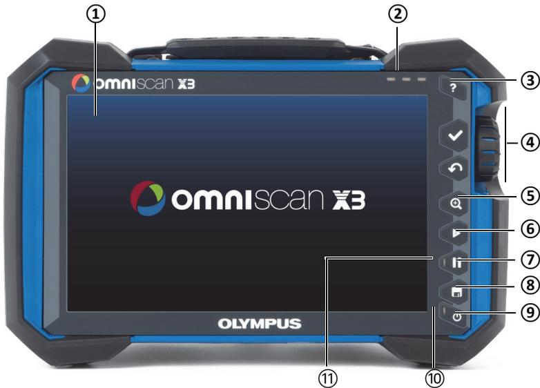
Figure 1-1 Front panel controls of the OmniScan X3 flaw detector
